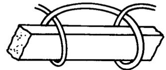
After the covering is attached, free the spars by cutting the restraining threads.
