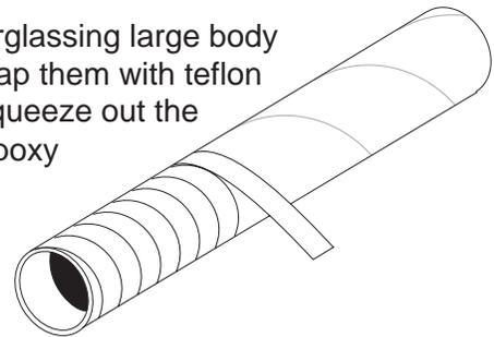
glass to give sufficient rigidity. Use epoxy sparingly. Epoxy doesn't add strength; only weight. I highly recommend the vacuum bagging technique to squeeze out excess epoxy resin from fiberglass cloths.
